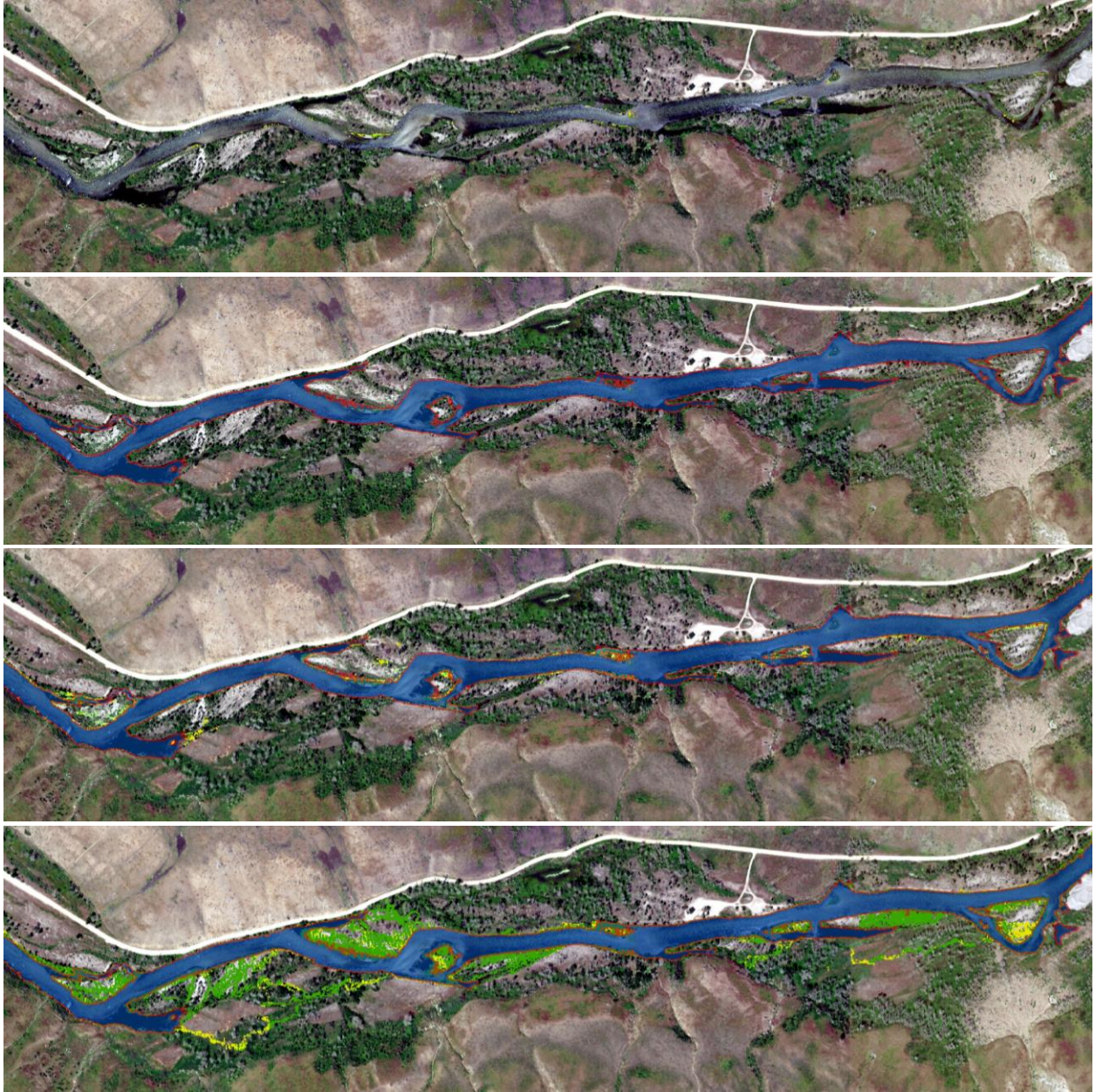
Figure 18. Simulated recruitment areas in Reach A for 2016 (top), 2016 with river mask of 45 m 3 /s discharge (second), 2017 with river mask (third), and 2016 planting option with river mask (fourth). Green is fully favorable conditions, yellow is partially favorable conditions, and orange is less favorable.
